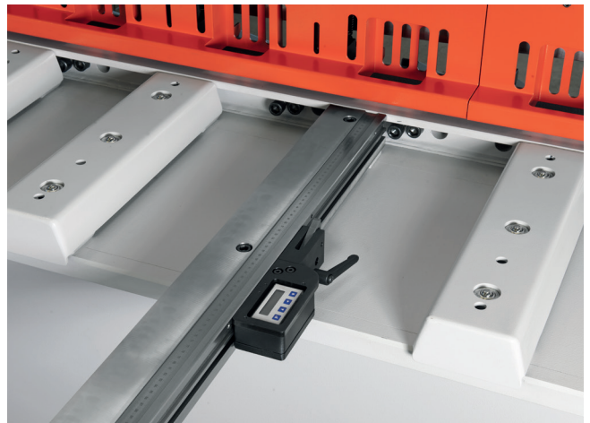
Disappearing front stop with digital LCD-display
